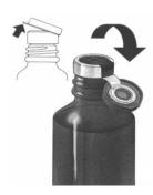
2. Tear off the sealing ring completely.
